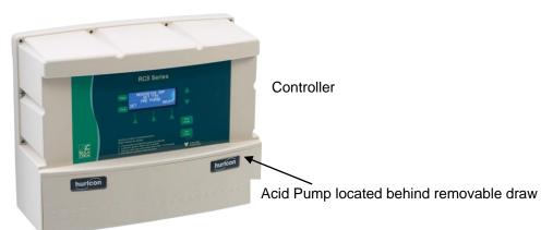
2.1 Mounting the Controller: Choose a location that is preferably out of direct sunlight, near the filter system. The controller should be located 1 metre above ground level to prevent rain splash back or sprinkler system damage to the underside of the controller. The controller must be mounted on a vertical surface/wall. If mounted on a post, a flat sheet 20mm larger than the controller housing must be used.
